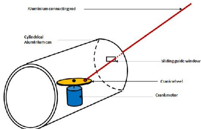
**Figure 7: Fish Core, Crank Motor, Crank Wheel and Connecting rod Assembly.**
