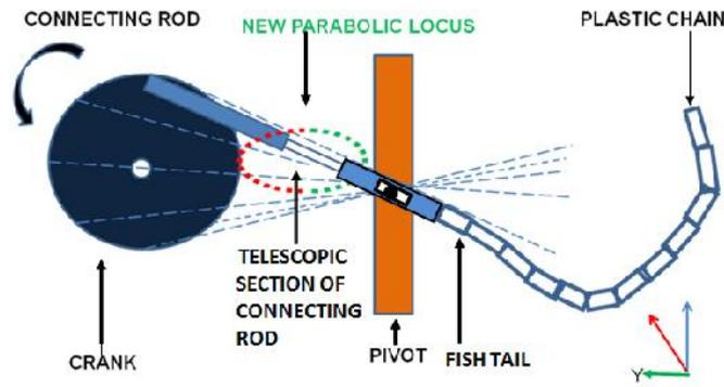
**Figure 5: Connecting ROD Showing Telescopic Section Attached to Crank.**
